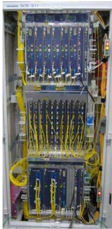
Fig. 5 External appearance of optical protection equipment
