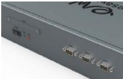
Side A - Detail of CFast slot , serial ports and main power push button switch. APO or ATX selection.
