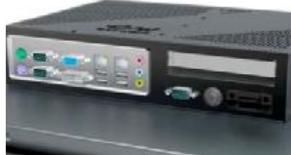
MITX version. Variety of Atom and i-core CPUs FANLESS and FAN Accessible dual slot bay 2,5" 2 independent LANs PCI / PCIe Slot
